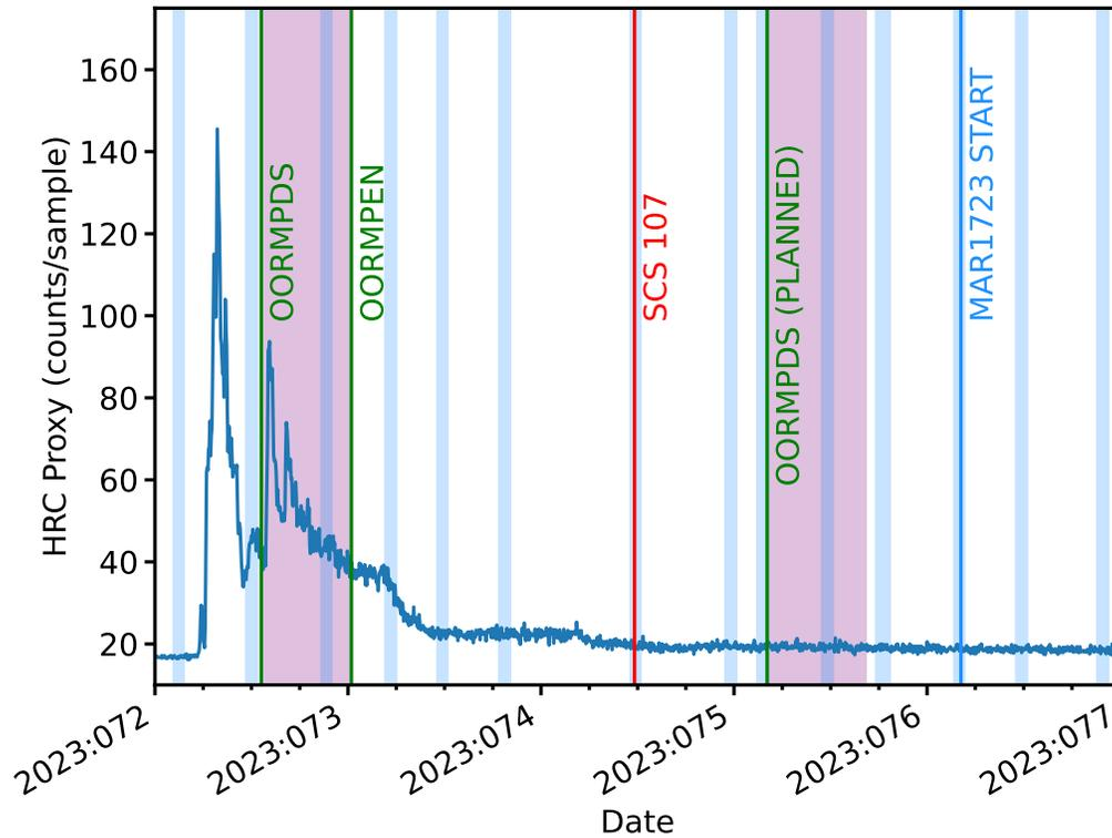
Figure 5: The HRC Shield proxy during the storm. Shaded regions and vertical lines have the same meaning as in Figure 1. Throughout the entire storm, this value was very far away from the trigger value of 245.
