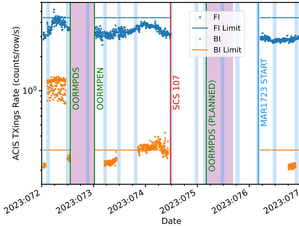
Figure 3: The txings plot for 2023:072-2023:077 (March 13-18). Blue is for FI chips, orange is for BI. The horizontal lines are the increasing values trip thresholds for each type of chip. Shaded regions and vertical lines have the same meaning as in Figure 1. Despite the txings values being above the thresholds for some time, the algorithm did not trip since the data were not monotonic.
